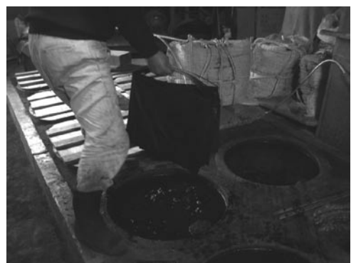
Fig. 5: Mr. Noguchi soaking the fabric in the dye-bath and checking the result.
