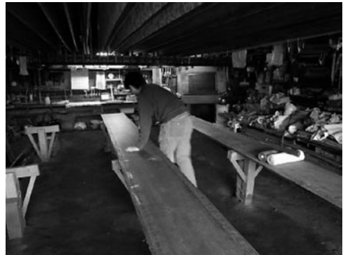
Fig. 2: Mr. Noguchi's son cleaning the long-board before laying the fabric.
